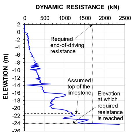
Figure 6 Determination of the expected pile toe elevation for a single test pile
