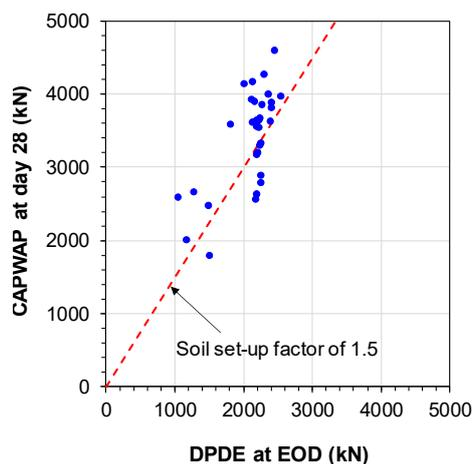
Figure 8 Soil set-up factor.
