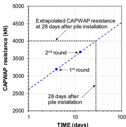
Figure 7 Example of CAPWAP resistance extrapolation.
