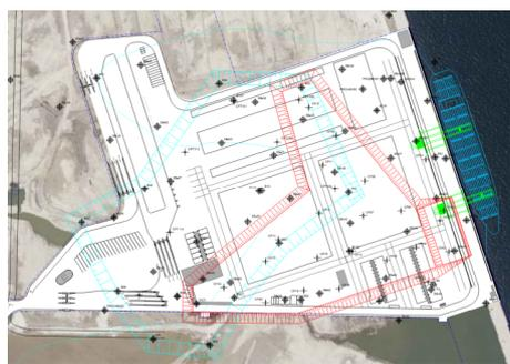
Figure 2 Construction site with the assumed location of the pre-consolidation (marked with red) and the approximate area of gyttja-membrane (marked with light blue) [3].
