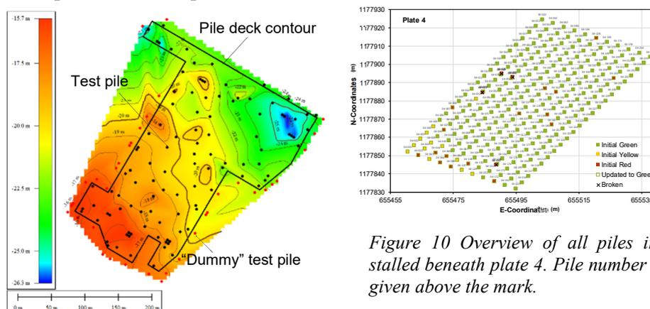
Figure 9 Expected pile toe elevation heat map.
