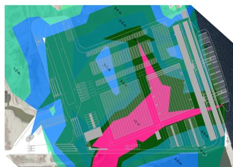
Figure 3 Variation of gyttja thickness at the construction site [3].
