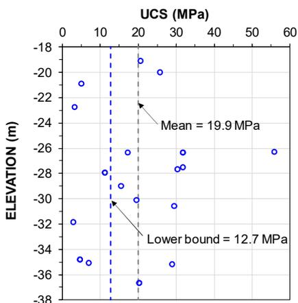
Figure 4 Unconfined compression strength of limestone.
