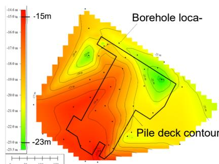
Figure 5 Top of limestone elevation with the pile deck contour and location of the boreholes.
